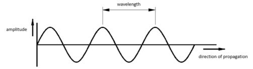
**Figure 4.** Waves – Amplitude and wavelength.
